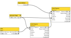
Sequence #1 gets started by a Trigger configured as "TwilightAm". Another Trigger is configured as "TwilightPm" and stops Sequence #1 and starts Sequence #2". Both Sequences are controlled with a Fader on the input Opacity, which is Brightness here.
