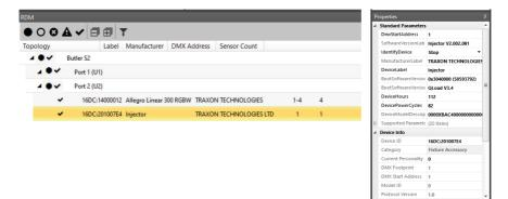
Configure the properties that effect the addressing. It is device-dependent which RDM properties these are and how to. The settings are immediately effective. Two examples for different devices to edit the DMX start address. Traxon Allegro Dot: First, enter a *LockState* in which *Enable Autoaddressing* and
