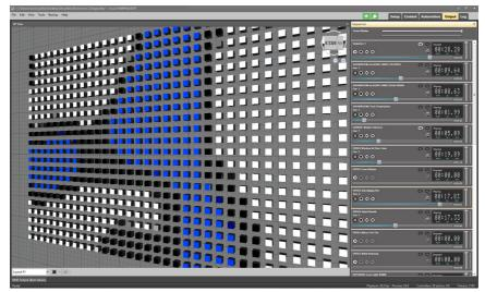
In the center, there is a preview of the currently running and viewed Layout. If there are several Layouts, you can select the one to view. In the Preview area, you can zoom in and out with the mouse wheel. Below the Output view, the DMX data is displayed. You can select either byte values or raw RGB. Selection is made with the two tabbed areas below the DMX Output window.
