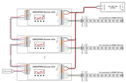
2.2) Total load of each LED receiver is over 10 A
