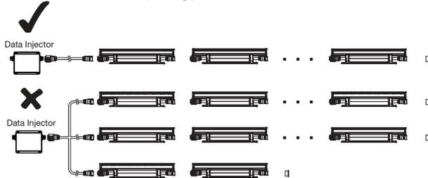
3. Each data injector can connect up to 32 fixtures regardless of fixture length.
