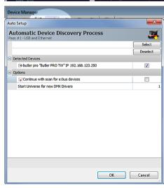
Using this device setup dialog you can set the DMX universes as well as the required RDM feedbacks for the channels of the Butler PRO DC
