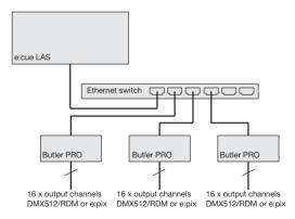
Use standard CAT5 RJ45 Ethernet cabling between server, switch and Butler PRO DC. Connection without Ethernet switch and with an Ethernet cross cable is not recommened. To connect DMX using a XLR5 type plugs, please use a adaptor cable, item number 40005, available as accessory or contact your nearest e:cue distributor for a suitable adaptor cable.
