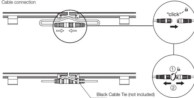
If you do not hear "click", rotate the spring loaded lock nut manually (in opposite direction to loosening) to ensure that the connectors are properly mated and tightened.
