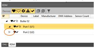
7. Click the triangle arrow and the list will expand revealing all of the detected devices on the output port of the output device.
