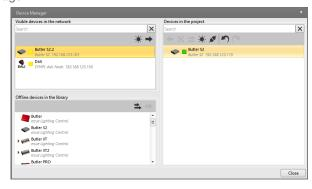
Enable RDM mode for the output device by right clicking on the output device and select Enable RDM.
