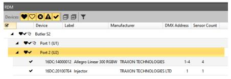
8. Click on an RDM device, here the Injector. Now its properties are displayed in the Properties tab on the right hand side of the screen.
